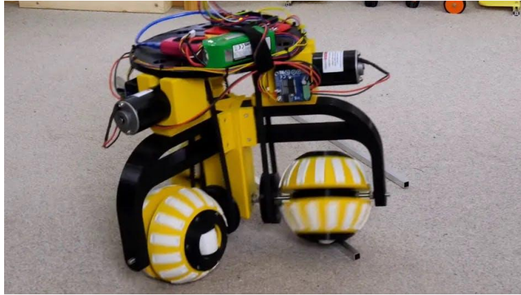
Figure 2.17 Example of robot using omnidirectional locomotion with three spherical wheels.
