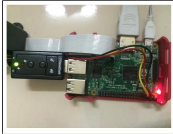
Figure 6.7: USB Sound Card connection with Raspberry Pi
