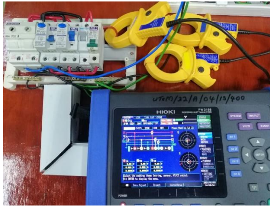
Figure 3-15 Power Quality Analyzer Used In The Project
