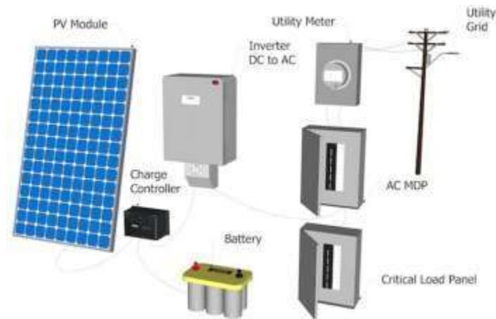
Figure 2. 3 The connection of the Bimodal PV System
