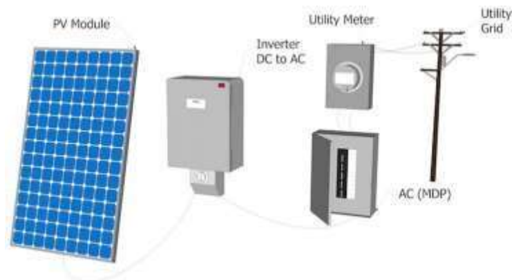
Figure 2. 2 The connection of the Utility Interactive PV System
