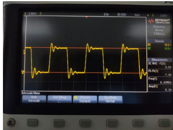
Figure 4.17 Output waveform at Oscillator, LTC1799
