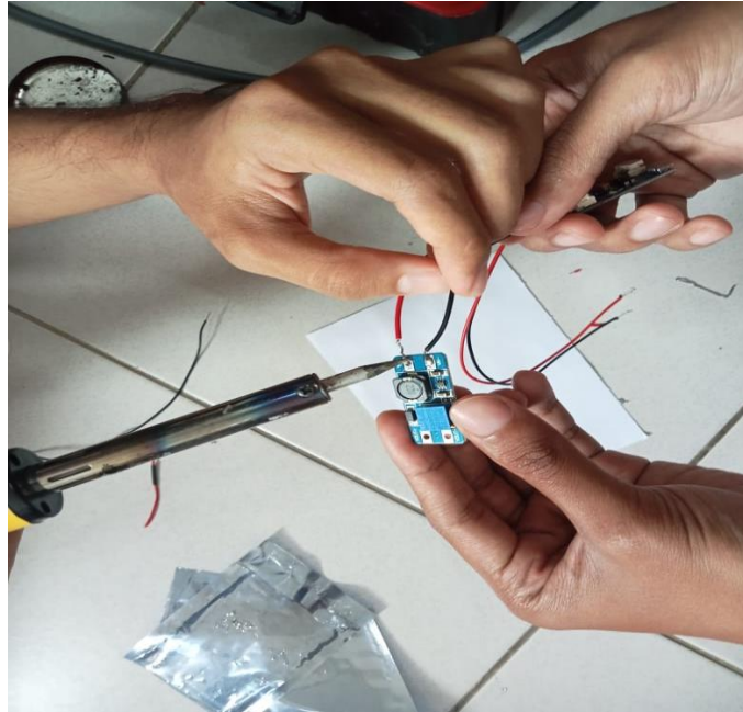
Figure 3.14 Make connections from solar to charge controller and to step up converter
