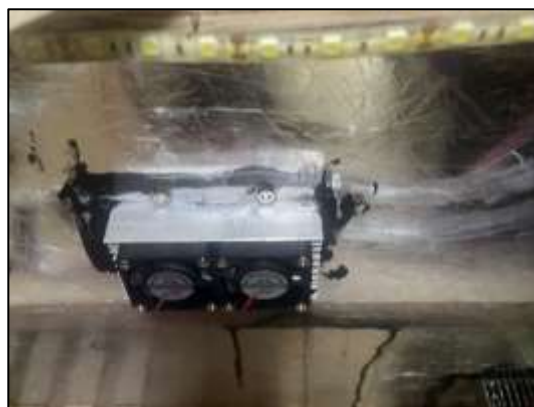
Figure 3.36 Water Cooling System Cool Down the Greenhouse Temperature
