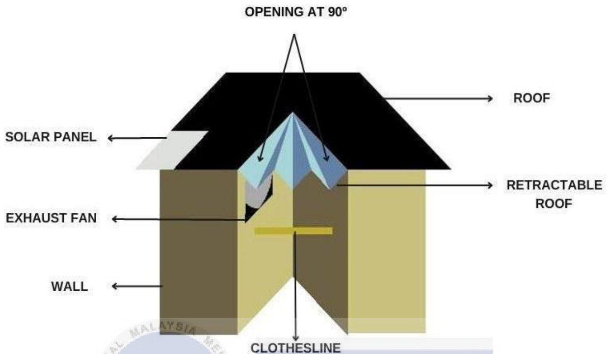
Figure 3.1 View when the roof in an open state at 90°.
