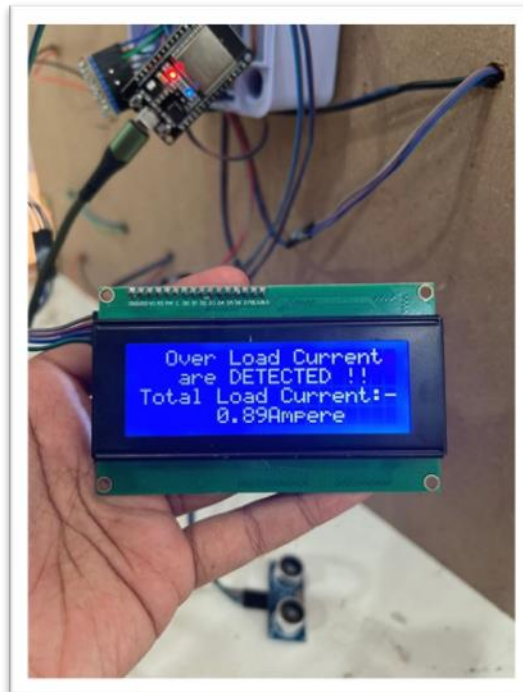
Figure 4.6 Example of overcurrent situation.
