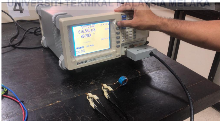
Figure 3.8 : Inductance connection to LCR meter
