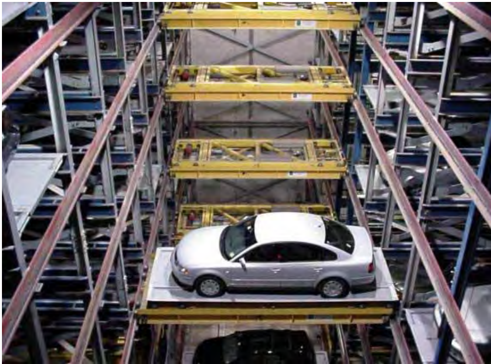
Figure 2.6 : Vehicle is transported on pallet using carrier and lift
