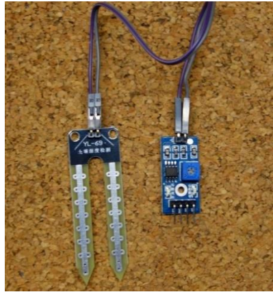
Figure 2.2 Soil Moisture Sensor YL-69: Electronic board (right) and probe (left)
