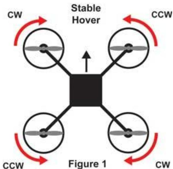
Figure 3.7: The rotation of propellers direction in quadcopter
