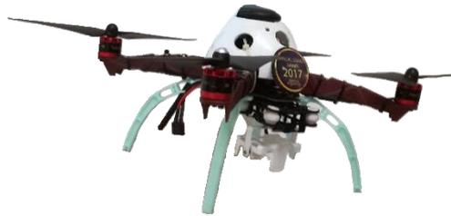
Figure 6.2: Assembled Arducopter
