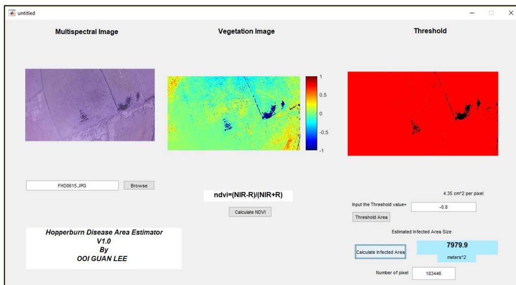
Figure 6.34: The testing result of image 615
