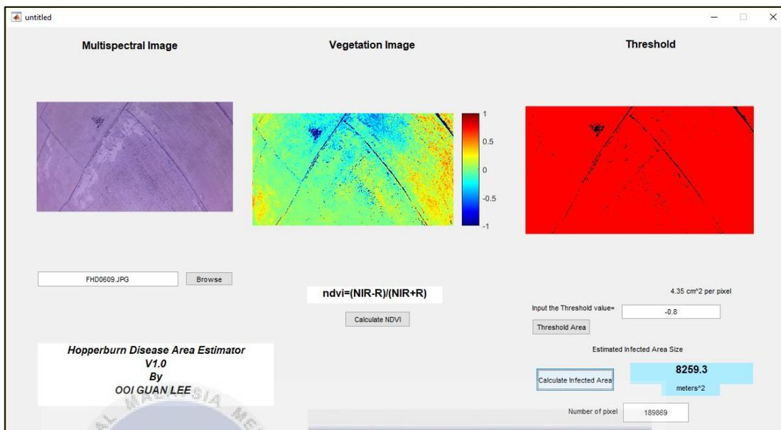
Figure 6.29.: The sample result of processed image in GUI
