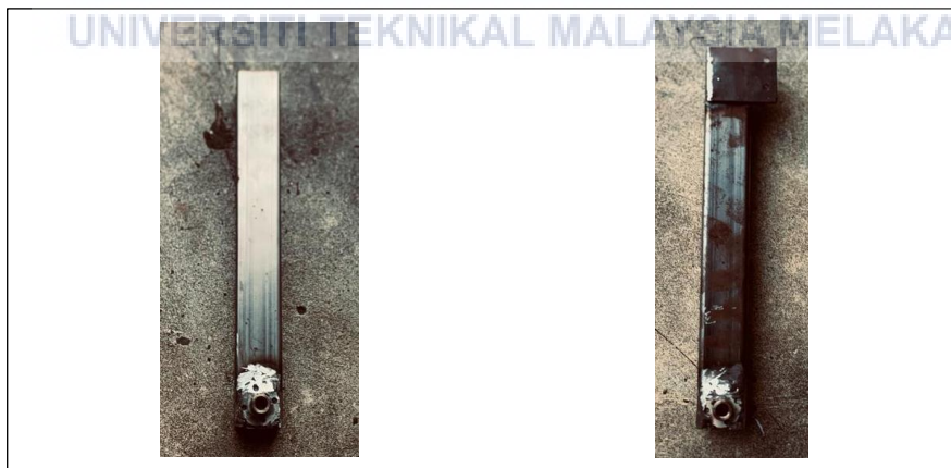
Figure 3.8 A piece of aluminum as the supports for the hanger
