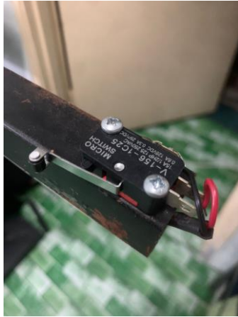
Figure 3.13 Limit switch for motor 3
