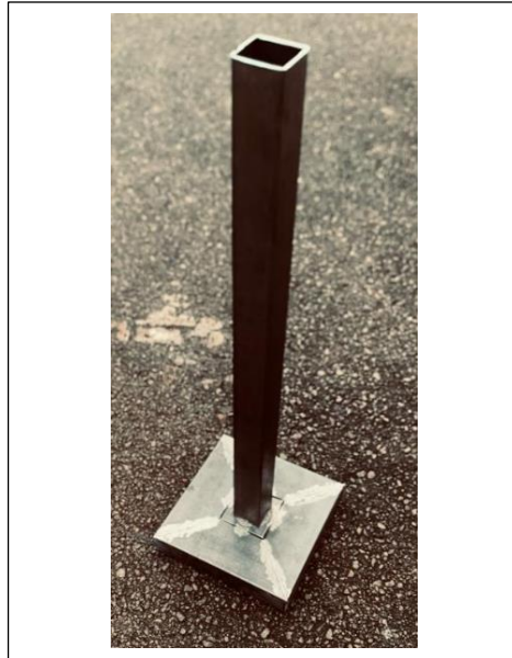
Figure 3.7 Combining base and the hollow stand
