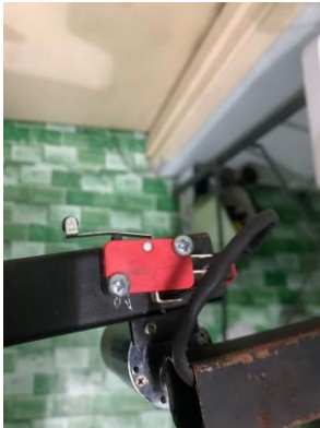
Figure 3.12 Limit switches for motor 2
