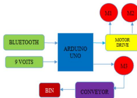
Figure 2.7 Block diagram of the proposed system[14]
