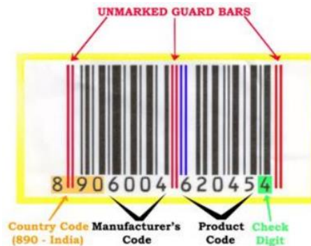
Figure 2.5 Components of a barcode
