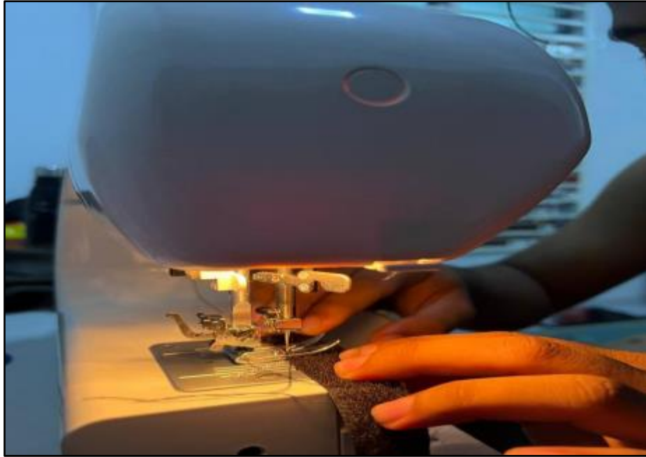
Figure 4.7 Sewing Velcro Tape onto Arm Exoskeleton Cuff
