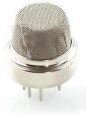
Figure 2.16 MQ-2 Gas Sensor detection
