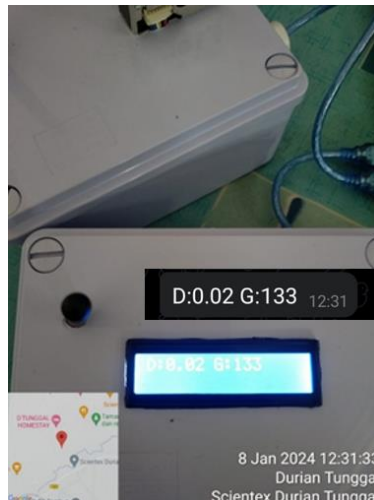
Figure 4.14 LCD screen and Telegram notification when gas no detected
