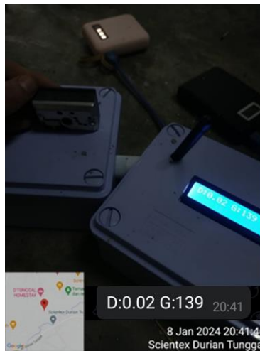
Figure 4.12 LCD screen and Telegram notification when dust no detected
