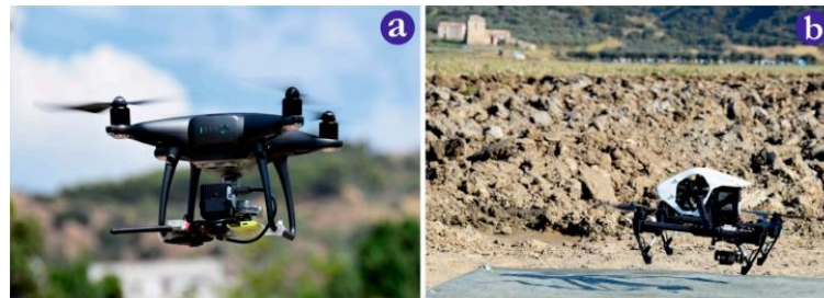
Figure 29 a, b DJI Phantom 4 pro & DJI Inspire both equipped with a FLIR uncooled thermal camera
