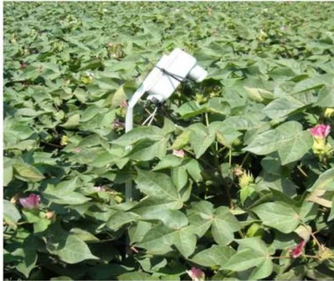
Figure 31 Cotton plant canopy temperature measured with an infrared thermometer
