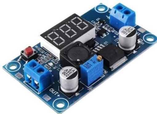
Figure 3.10 An LM2596 Voltage Regulator
