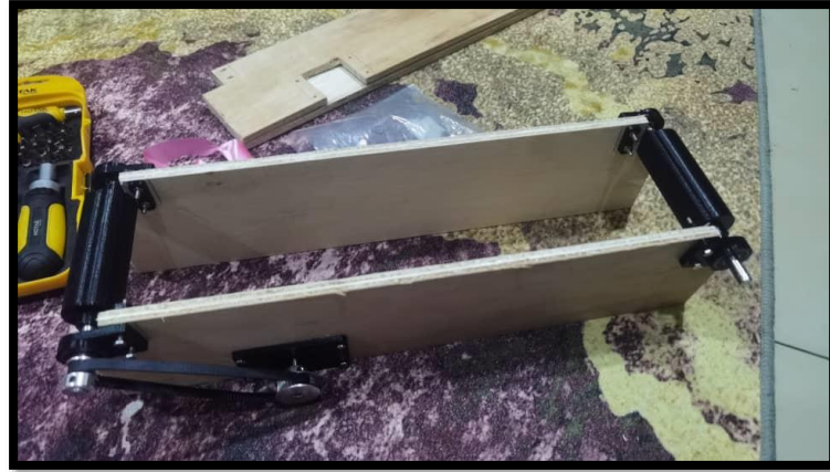
Figure 4.4 The Frame of the Body Conveyor
