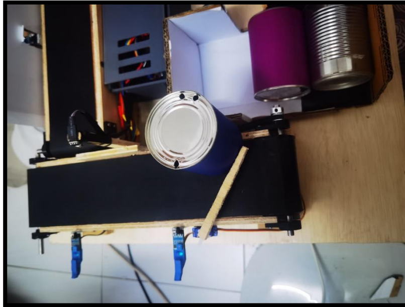
Figure 4.8 The Servo Operated to seperate the defective cans
