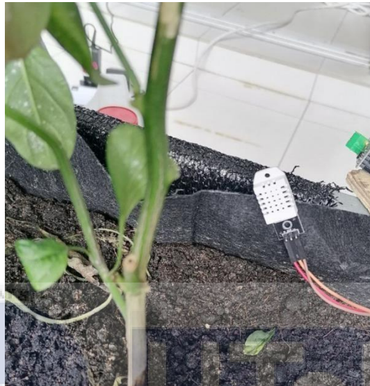
Figure 3.7 Temperature And Humidity Sensor Setup
