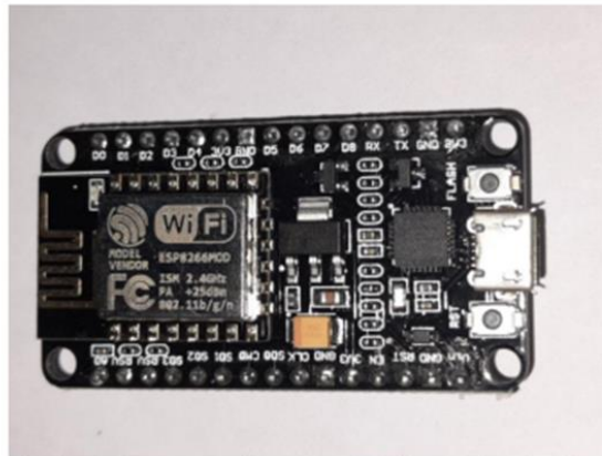
Figure 2.7 NodeMCU ESP8266 board with Wi-Fi solution
