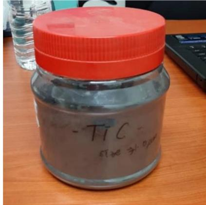
**Figure 3-5 The Compound of Titanium Carbide Powder**
