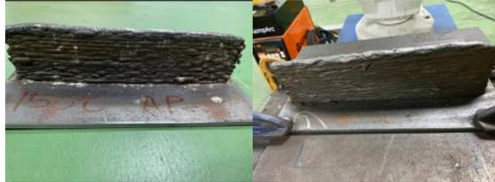
**Figure 4-1 Surface morphology of alumina oxide powder left side, and titanium carbide powder right side**
