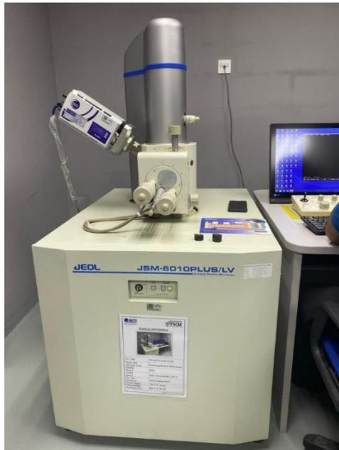
**Figure 3-19 JEOL JSM-6010PLUS/LV SEM machine**
