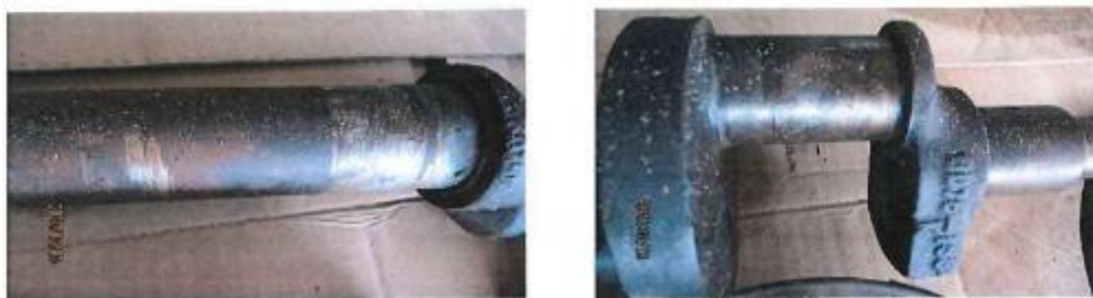
Figure 3-2 Picture failure of crankshaft
