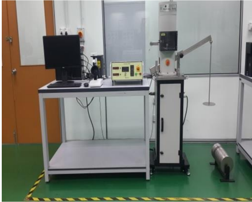
Figure 3.9 Koehler K93190 four ball tester
