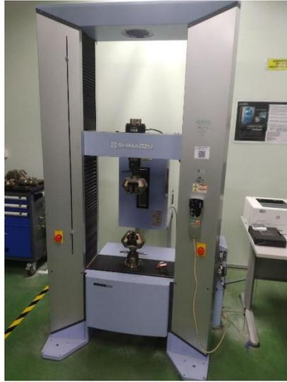
Figure 3.14: Shimadzu Autograph AG-100 KNG Universal Testing Machine
