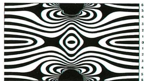
Figure-8 Photo elastic pattern: The extreme fibres of the beam away from the notches have 6 units of stress; in the bottom of the notch the stress is greater than 11 units
