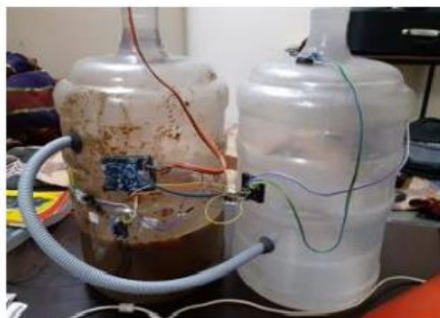
Figure 6 the hardware setup for smart sewage monitoring system
