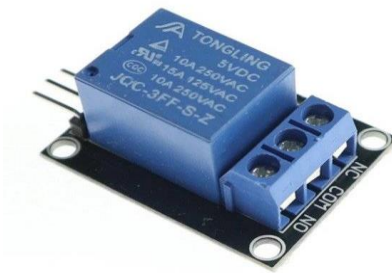
Figure 2.20: 1 Channel 5V Relay
