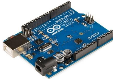
Figure 2.11: Arduino UNO R3
