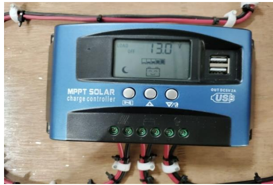
Figure 4.6: Main Display of MPPT Solar Controller
