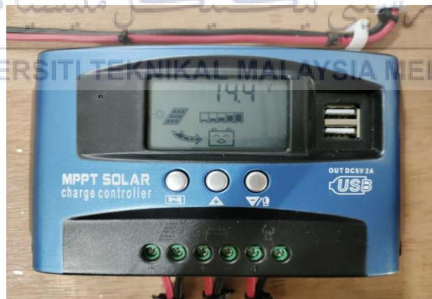
Figure 4.7: Over Charging Protection Setting Display
