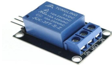
Figure 3.7: 1 Signal Relay (5V)
