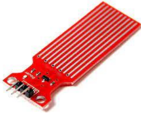
Figure 3.8: Water Level Sensor (WH-038)
