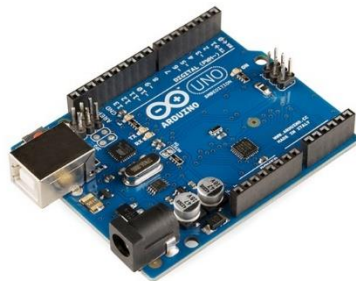
Figure 3.9: Arduino UNO R3
