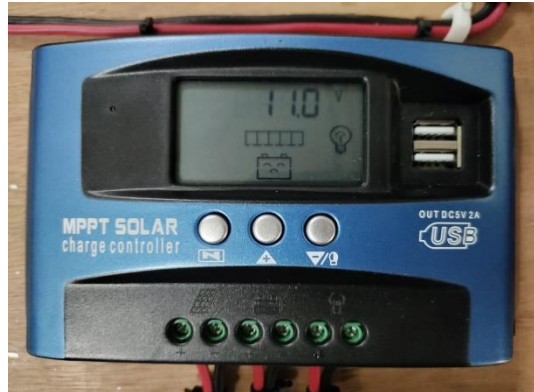
Figure 4.8: Over Discharging Protection Setting Display
