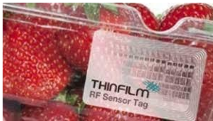
Figure 4.4: RFID Tag on food packaging
