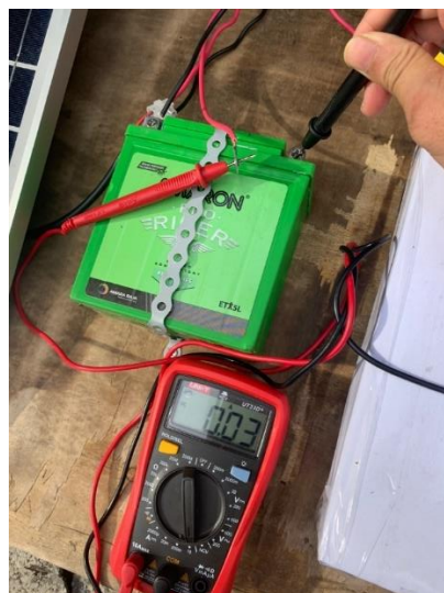
Figure 4.14 Current from Solar Panel to Battery
