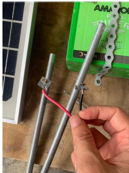
Figure 4.8 Battery Terminal from Screw and Used Iron
