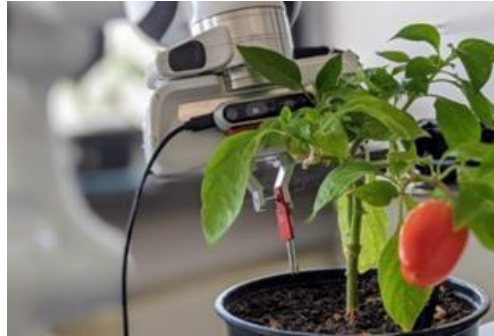
Figure 2.1: The robot performing soil moisture measurement[1]
