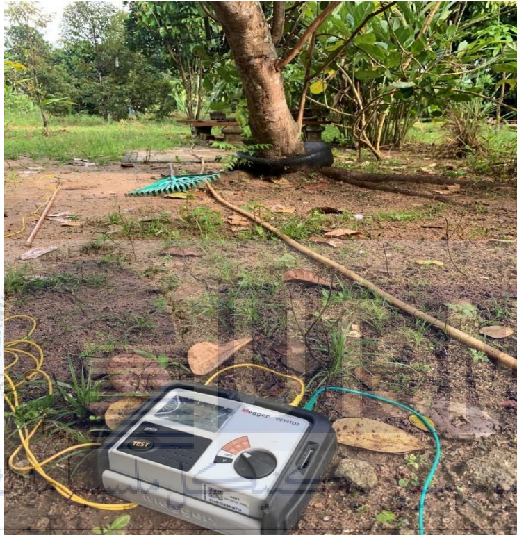
Figure 4.18 Measure earth resistance when moist soil
