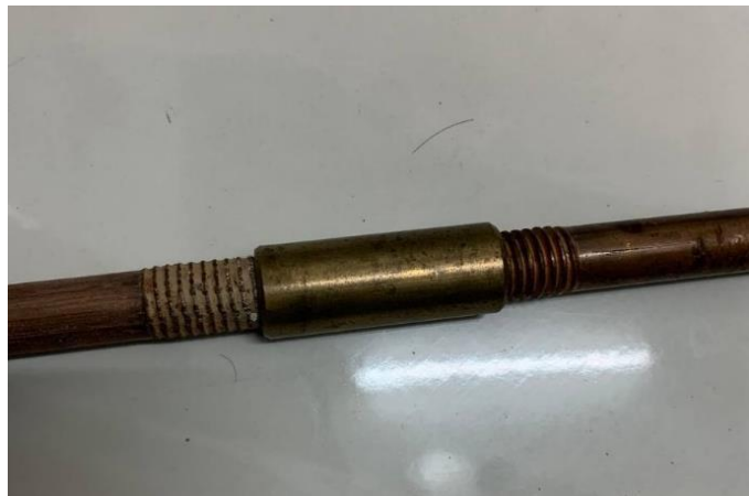
Figure 4.4 Rod attached to another rod using earth coupling.
