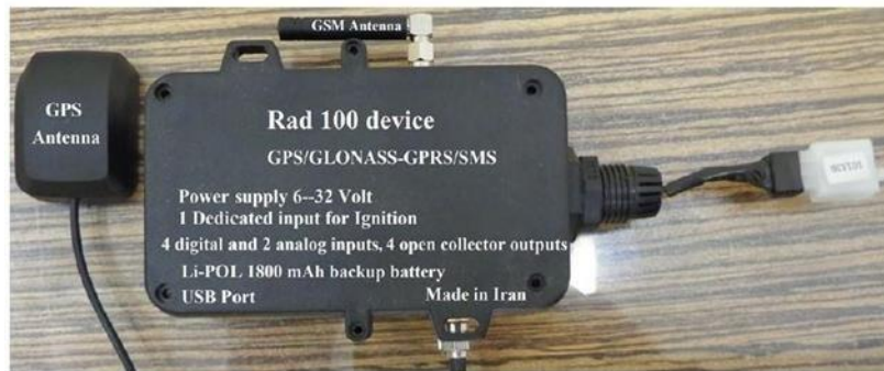
Figure 2.4 Rad100 Hardware and Box with Embedded Rad100 Tracker
