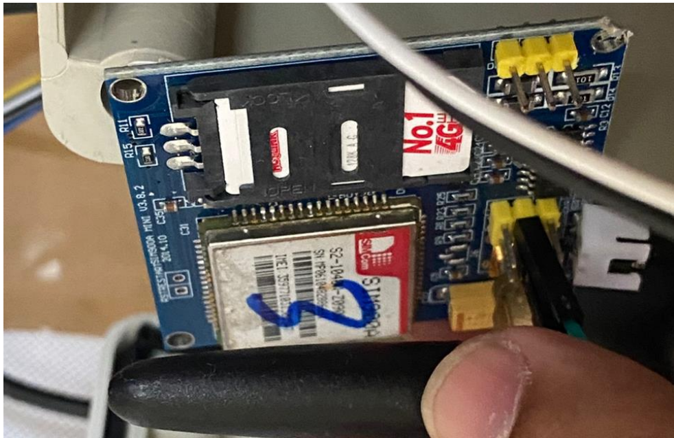
Figure 4.9 GSM 900A inserted with Maxis simcard.
