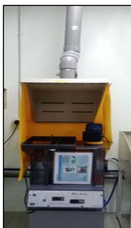
Figure 7. 3:PCB Developer Machines
