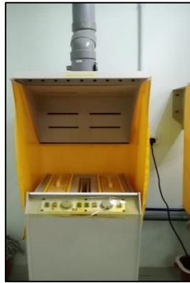
Figure 7. 5: Photoresist Stripper Machines
