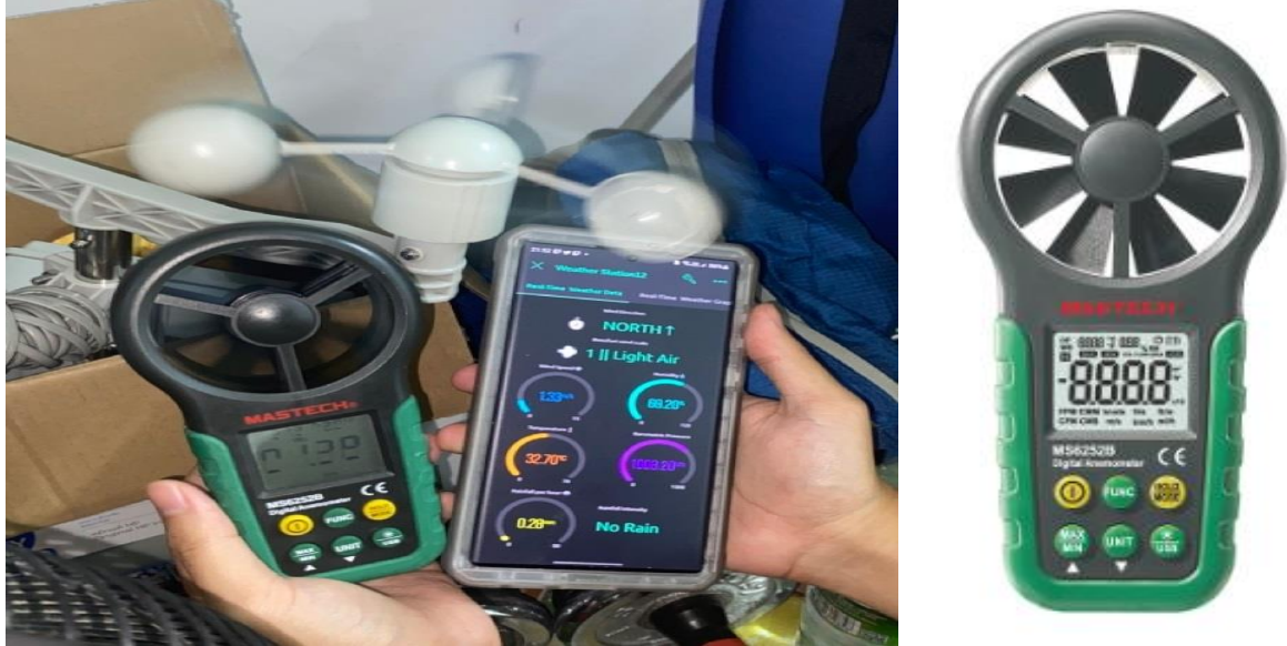
Figure 4.8 Verify project wind speed against Mastech digital anemometer
