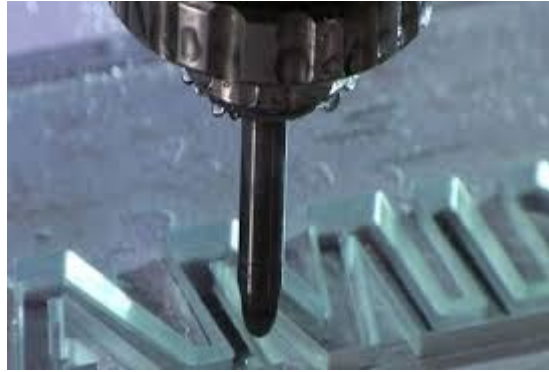
Figure 2.8 Glass cutting using AWJ (Goldberg, 2018).
