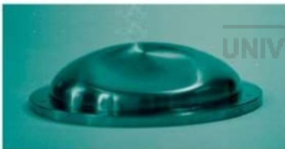
(a) Buckled/Collapsed storage tank
