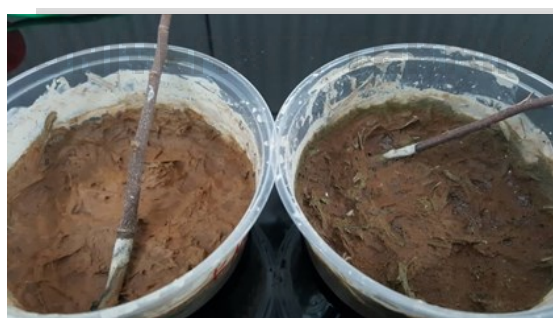
Figure 1: Decomposing of paddy straw and stubble with a decomposing inoculant after one month shows decomposed leaves (left sample) and a non-treated sample with intact leaves structure (right)
