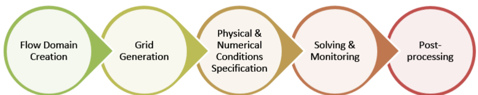
Figure 1 Typical steps of CFD modelling process
