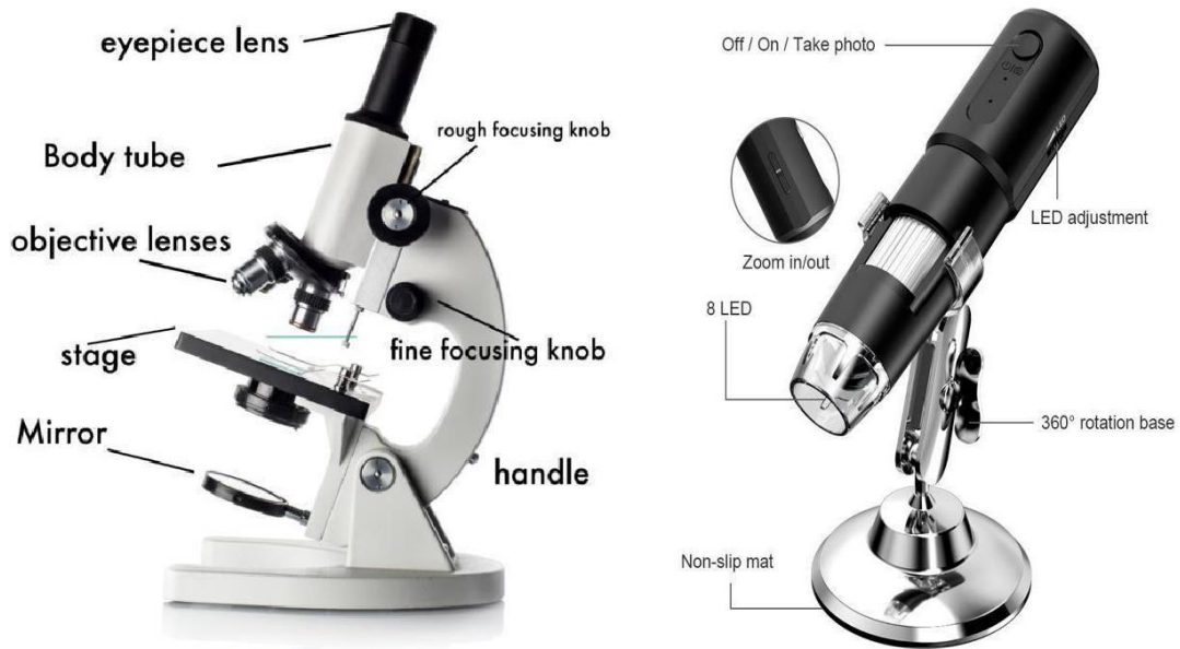
Figure 1.2: Components in Normal Microscope and Portable Microscope (RS Science , n.d.)
