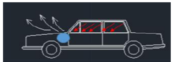
Figure 4: Reversed blower vacuum releases the hot air that trapped inside car cabin.
