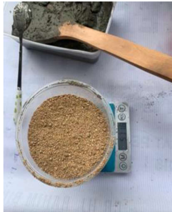
b) All the prepared materials are weighted.
