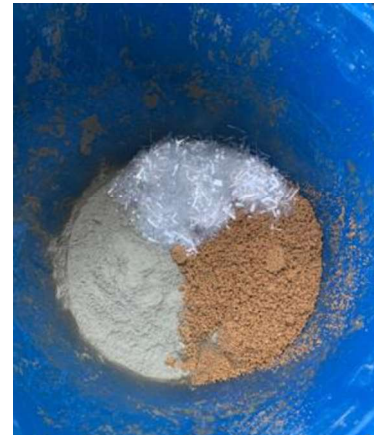
c) The weighted materials are placed in a pail for dry mixing.
