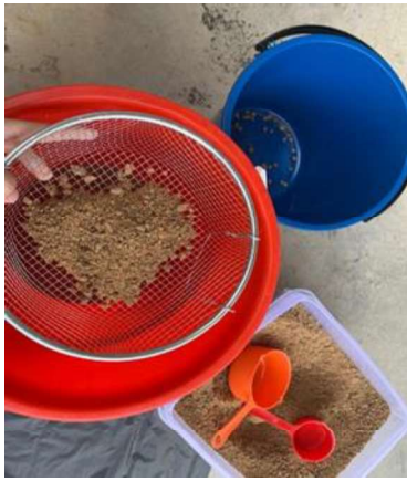
a) The cement and fine sand are sieved.
