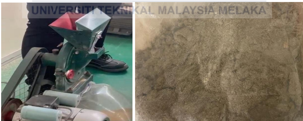
Figure 3.6 Scratcher machine and pineapple leaf powder
