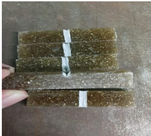
Figure 3.16 V-notch of the specimen
