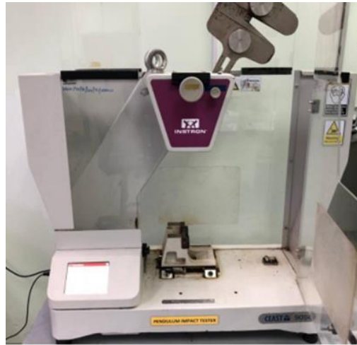
Figure 3.24 The charpy impact INSTRON CEAST 9050 machine
