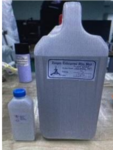
Figure 3.10 Polyester resin and hardener (BUTANOX M-50)
