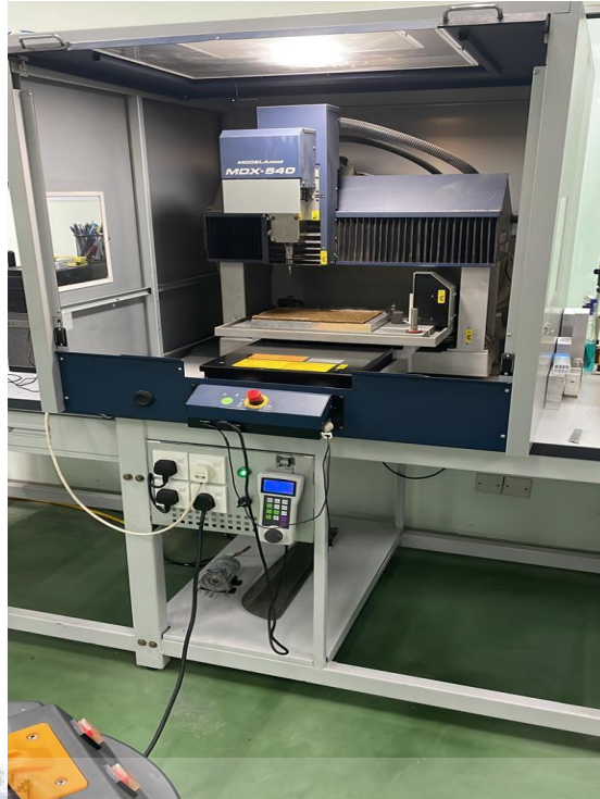
Figure 3.23 CNC router machine model MODELA PRO2 (MDX-540)
