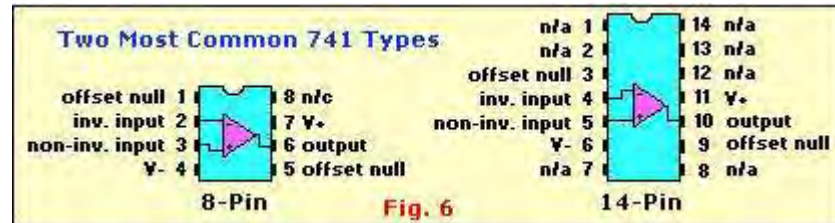
Figure 4.3.5: 741 Op Amp pin functions
