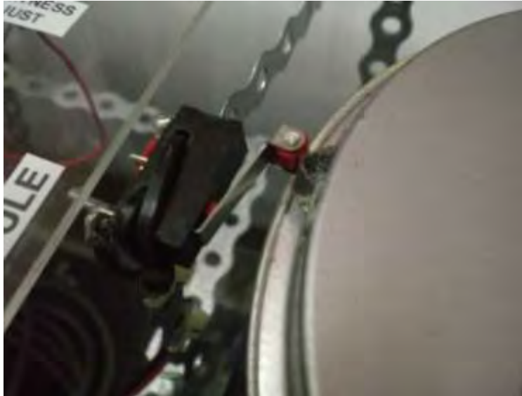
Figure 4.2.5(c): Limit switch and triangular marker
