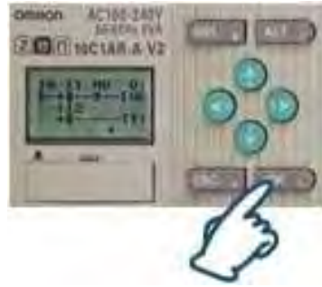
Figure 4.3.2(b): Programming the Omron ZEN
