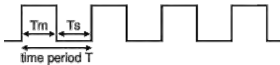
Figure 4.3.4(c): 555 Astable output, a square wave
