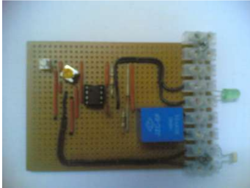
Figure 4.2.2(b): Assembled circuit for the Outdoor Lighting
