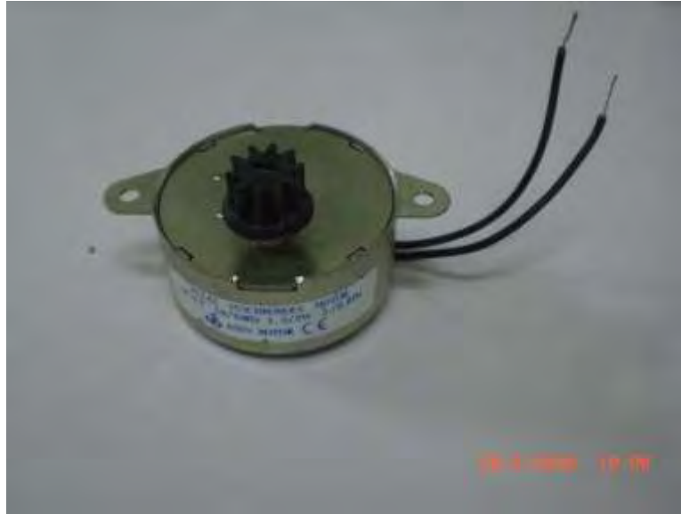
Figure 4.2.4(e): AC Synchronous motor used for platform rotation
