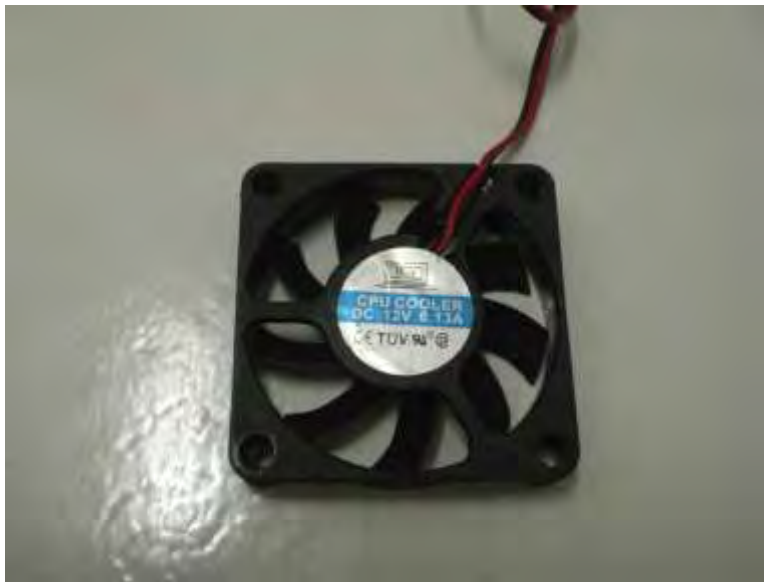
Figure 4.2.3(e): 12VDC CPU fan rated at 0.13A
