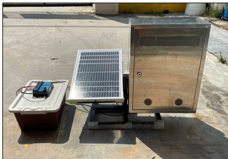
Figure 4.5 Hardware Development of Mailbox Notification System with Solar Battery Charging
