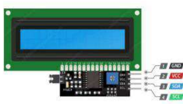
Figure 3.7 I2C LCD pinout
