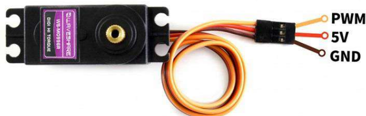
Figure 3.8 Servo Motor pinout
