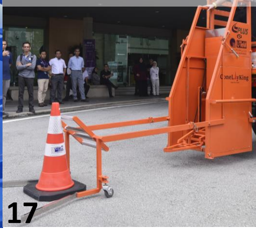
Development of a Semi-Automatic Cone Laying and Picking Machine for Maintenance and Emergency Use
