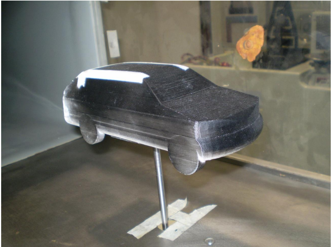
Fig 3.4 A model tested in wind tunnel
